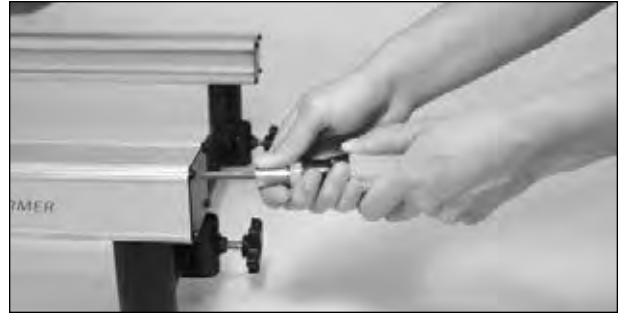
2. Using a Phillips screwdriver, remove stopper plates.
