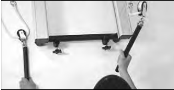
1. To remove carriage, remove pulley posts and place on the floor, on either side of the aluminum rails.
